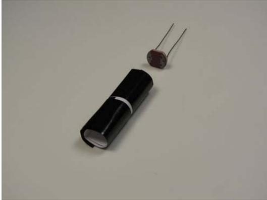
**Paper Tube Ready for Photoresistor**
