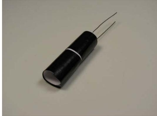
**Photoresistor Inserted into Tube**
